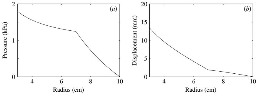
FIGURE 3. Complete occlusion: calculated values in parenchyma of (a) fluid pressure relative to subarachnoid pressure, (b) displacement when grey matter permeability decreased and stiffness increased.
