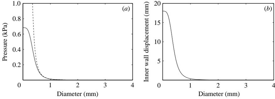
FIGURE 4. Effect of varying the aqueduct diameter,  $d$ , on pressure drop across the parenchyma and wall displacement. (a) —, pressure drop,  $p_g(C) - p_w(A)$ ; - - -, Poiseuille pressure drop for CSF flow through tube of diameter  $d$ , (b) inner wall displacement,  $u_w(A)$ .
