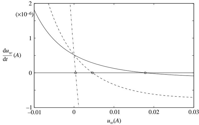
FIGURE 5. Phase plots for the wall displacement,  $u_w(A, t)$  showing a stable fixed point (encircled) for various aqueduct diameter:  $d = 0$  (—),  $d = 0.0005$  (- - -),  $d = 0.001$  (- · -).
