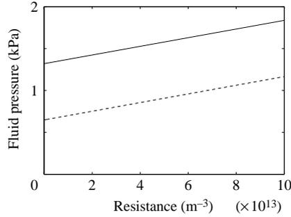
FIGURE 7. Effects of increasing the absorption resistance,  $R$ , on the ventricular pressure,  $p_w(A)$ , and subarachnoid pressure,  $p_g(C)$ .
