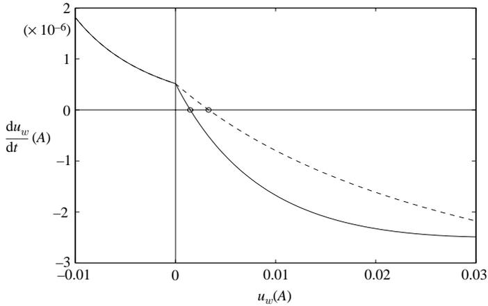
FIGURE 8. Phase plots of the ventricular wall displacement,  $u_w(A)$  with shunting showing a stable fixed point for ball on spring shunt (—) and for silicone diaphragm shunt (- - -).
