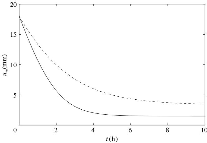
FIGURE 9. Time evolution of displacement,  $u_w(A, t)$  following introduction of shunt (a) (—) ball on spring shunt, (b) (- - -) silicone diaphragm shunt.
