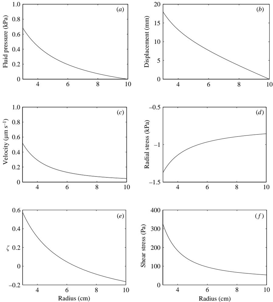
FIGURE 2. Complete occlusion: calculated values in parenchyma of (a) fluid pressure relative to subarachnoid pressure, (b) displacement, (c) superficial fluid velocity, (d) radial stress, (e) fluid increment, (f) shear stress.
